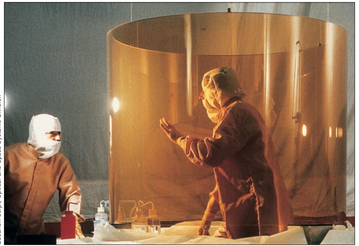
■ FIGURE 3-29 One of the cylindrical mirrors from the Chandra X-ray Observatory. Its inside is polished to reflect x-rays by grazing incidence.
